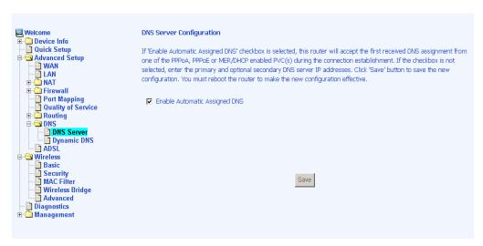
If you uncheck the *Enable Automatic Assigned DNS* checkbox, then there will be two additional fields—primary and secondary DNS server—to enter as seen below.
